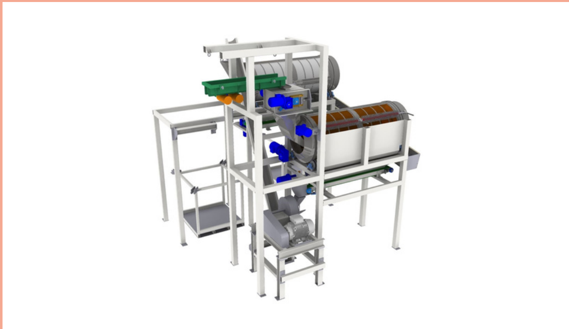
Preliminary design of the prototype for separating the biological membrane from the eggshell (MAINCER, S.L.).
