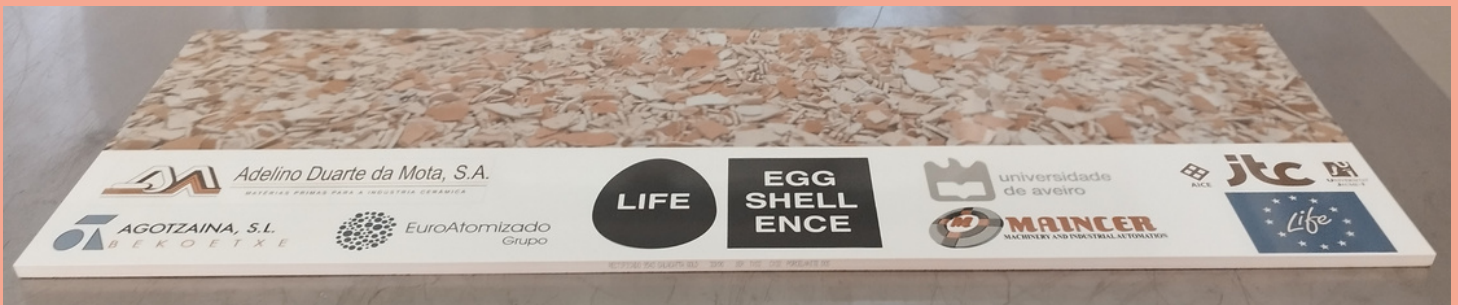
One of the tiles obtained with the atomized powder containing 5% bio-carbonate.
