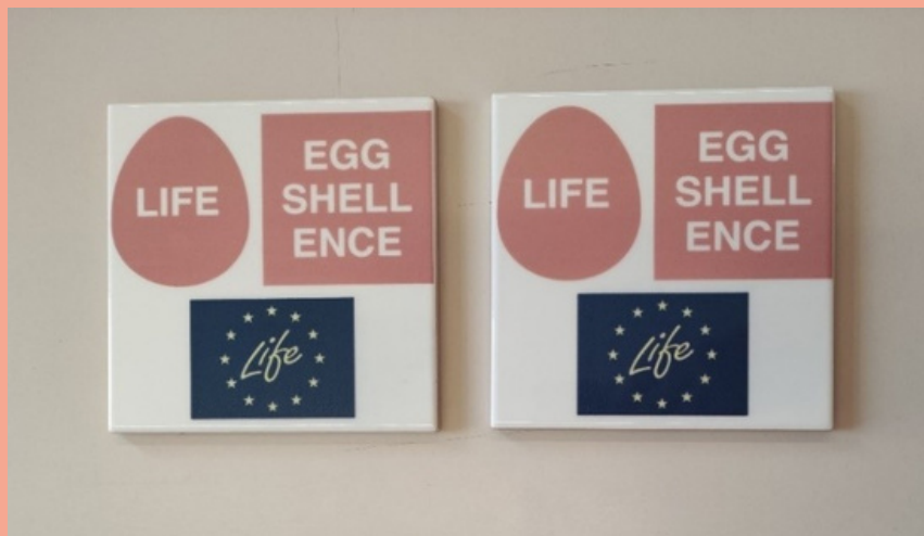
Tiles of 15x15 cm obtained with the standard composition (left) and with the composition with 5% of bio-carbonate (right).
