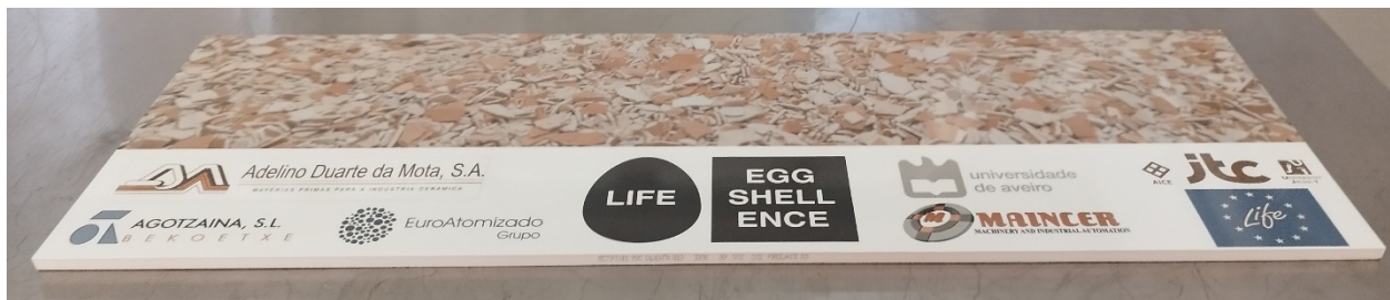
Figure 5. Earthenware tile produced industrially from a composition with 5% bio-carbonate.
