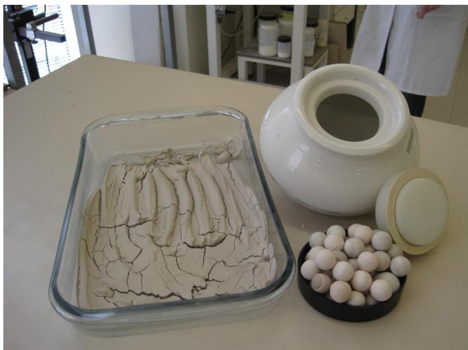
Figure 1. Laboratory milling of the compositions.
