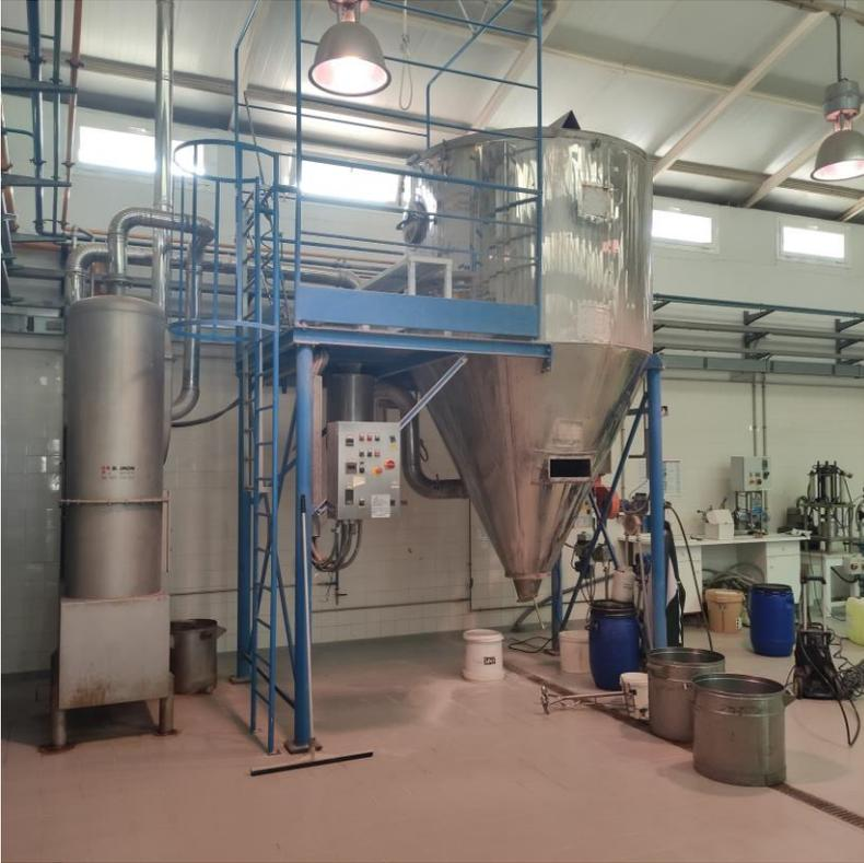
Figure 2. Spray-drier used for the preparation of the spray-dried powders.
