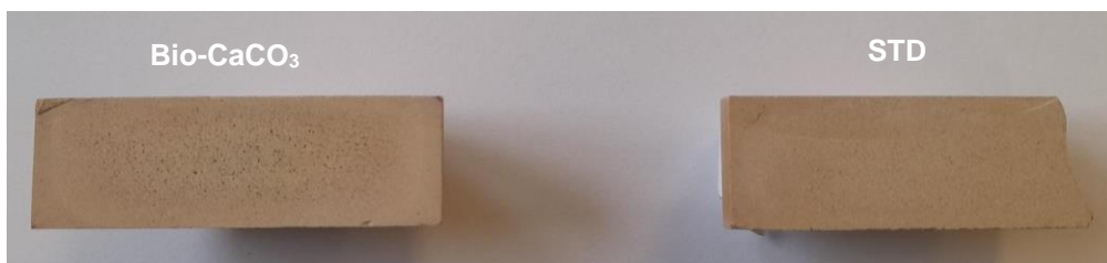
Figure 9. Tendency to black core formation.
