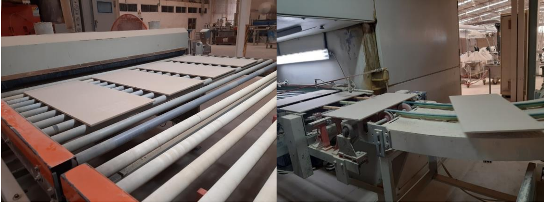
Figure 4. The pressed tiles dried and entering in the glazing line at about 85°C.
