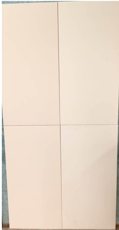
Figure 7. Fired wall tiles without glaze (left STD, right Bio-CaCO 3 ).
