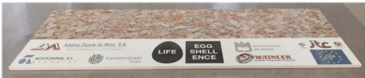
Figure 2. Specially decorated tiles obtained with the spray-dried powder containing 5% of bio-carbonate.
